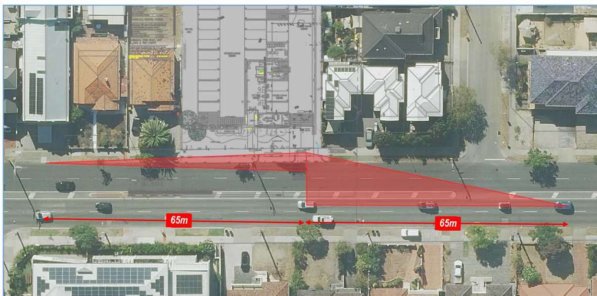
Figure 8: Sight Distance Check – Charles Street
