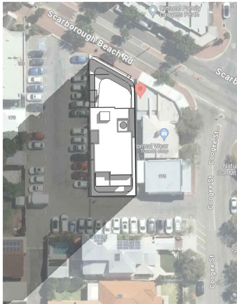
SHADOW DIAGRAM - 9am JUNE 21st NOT TO SCALE
