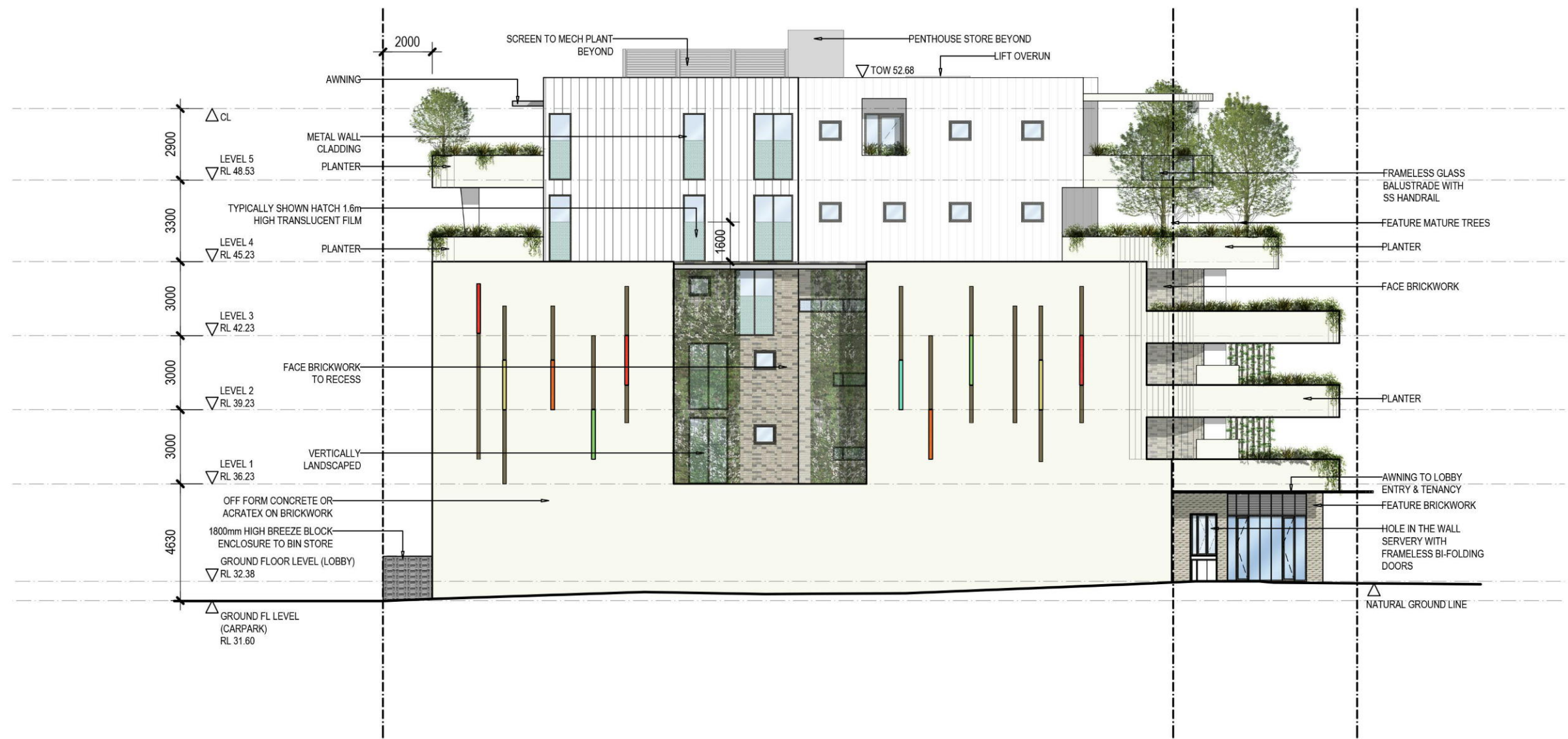
EAST ELEVATION SCALE 1:200
